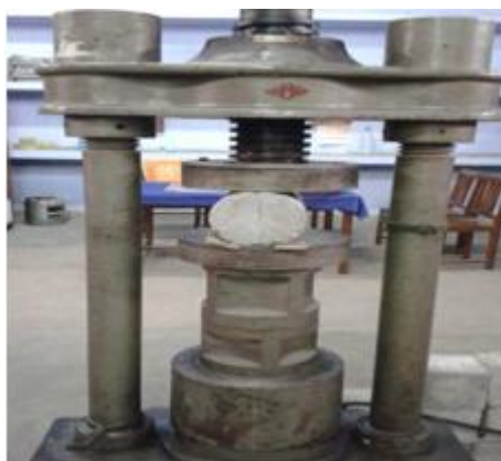
Fig. 2 Split Tension Test
